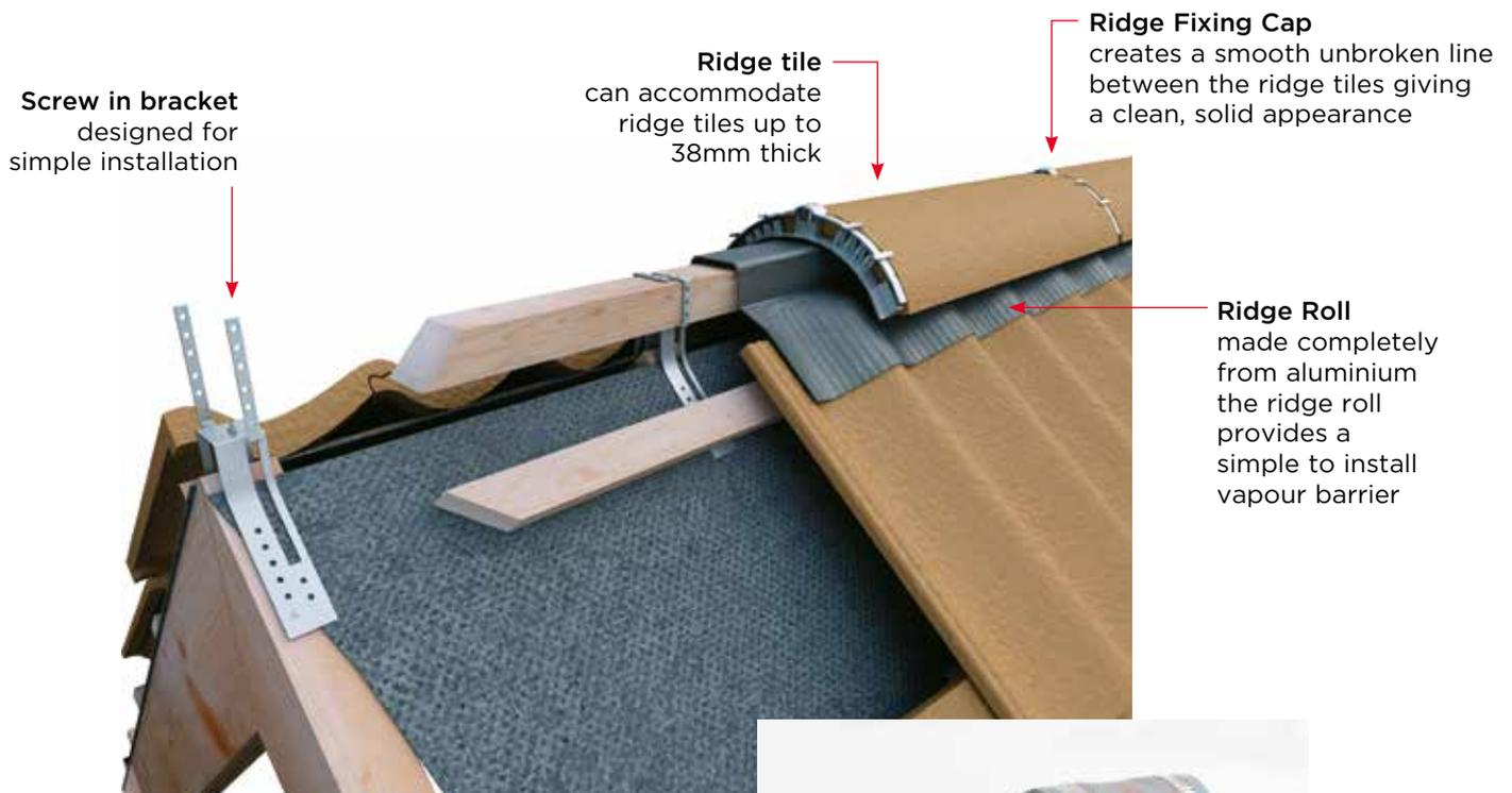
The Corovent dry fix system is supplied as a complete system with all the components to fix 6m of ridge.
